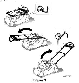
2. Unlock the upper handle locks and rotate the upper handle upward and lock it into a position that is comfortable to you (Figure 4).
